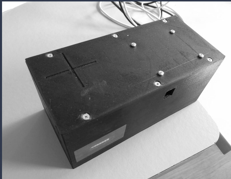
SPRM - Scintillator with PH32 chips Radiation Monitor
