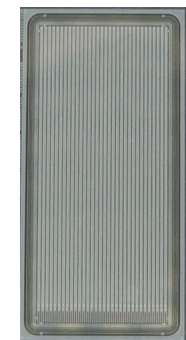
Four layers PH32 silicon strip telescope
